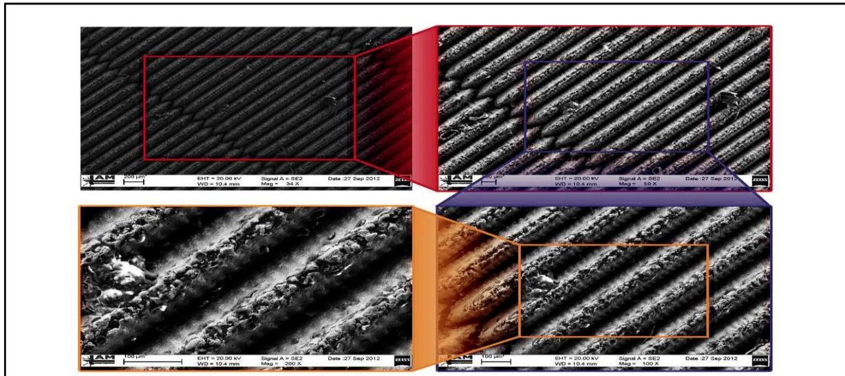
Fig. 5 SEM micrographs of laser beam machined hierarchical surface of cavity insert
