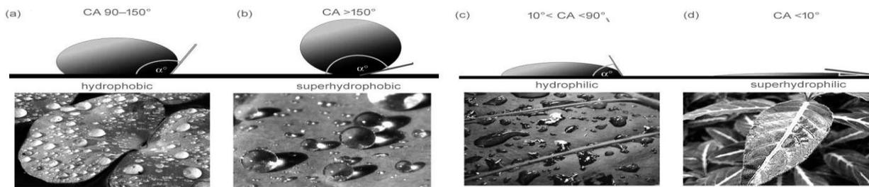
Fig.1. Four classes of surface wettability and representative leaves examples: a) hydrophobic, b) superhydrophobic, c) hydrophilic, d) superhydrophilic [3]
