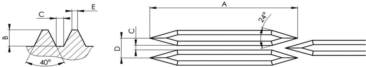
Fig.4. Design of hierarchical surface structure for replication by laser beam machining
